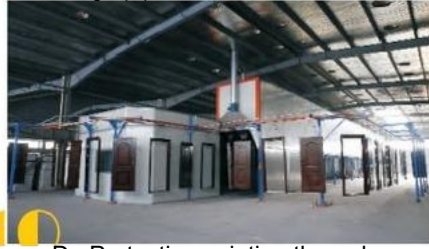
Do Protective painting through automatic painting system
