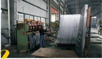
Open the holefor the accessories
