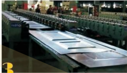
Adjust the steel sheet size by metal work stamping and folding system
