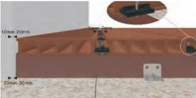
For plastic clip No.1, side-side gap between decks is 6-7mm
