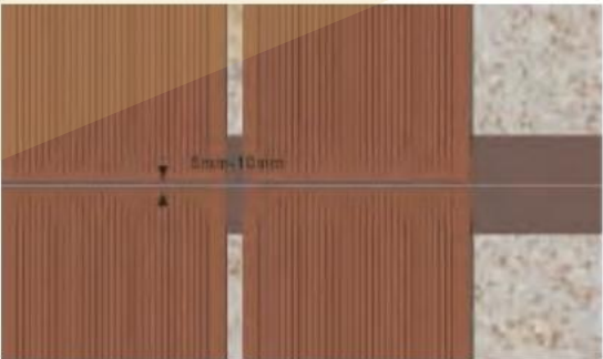
End*end gap of decks is 5-10mm
